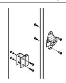
With the door in the closed position, position the strike/keeper on the pilaster and align the top so it is 1/2" (13mm) above the bottom of the latch slide bar. Using the strike/keeper as a template, mark the hole locations and drill Ø1/4" holes through the pilaster. Secure the strike/keeper to the pilaster with the #10-24 x 3/4" barrel nuts and #10-24 x 1" shoulder screws provided.
