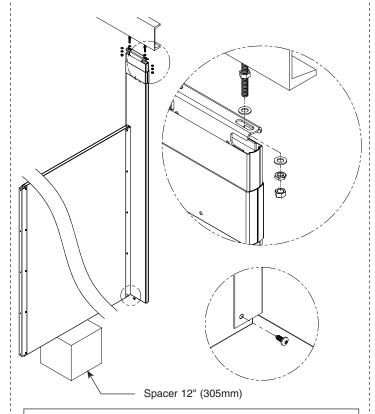
Using the bracket as a template, drill Ø3/16" holes through the panel at each panel bracket hole. Secure the panel to the bracket using the #14 x 5/8" stainless screws provided.
