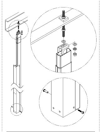
Using the bracket as a template, drill Ø1/4" holes through the pilaster at each pilaster bracket hole. Secure the pilaster to the bracket using the #10-24 x 3/4" stainless barrel nuts and #10-24 x 1" stainless shoulder screws provided.
