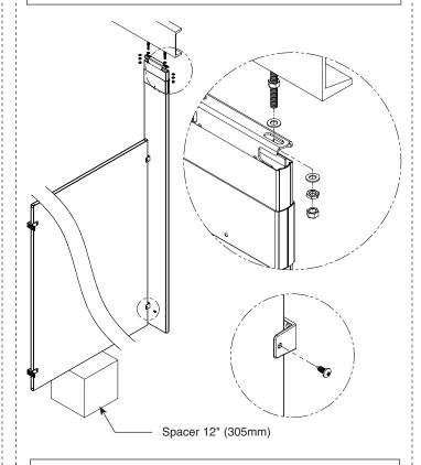
Using the bracket as a template, drill Ø3/16" holes through the panel at each panel bracket hole. Secure the panel to the bracket using the #14 x 5/8" screws provided.
