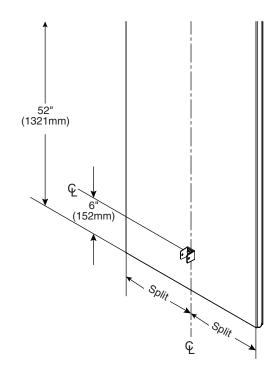
Measure 6" (152mm) and 52" (1321mm) up from the bottom of each pilaster and place a mark on the pilaster split centerline.
