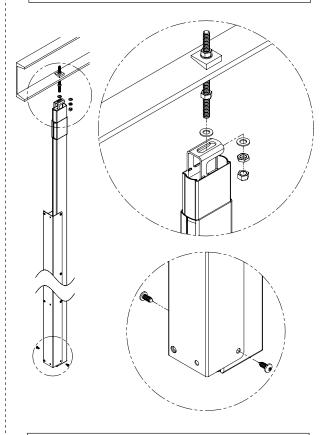
Using the bracket as a template, drill Ø3/16" holes through the pilaster at each pilaster bracket hole.
