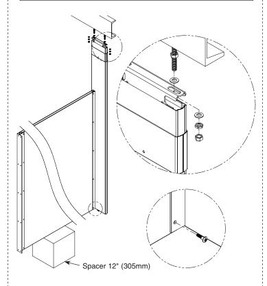
Using the bracket as a template, drill Ø1/4" holes through the panel at each panel bracket hole. Secure the panel to the bracket using the #10-24 x 3/4" stainless barrel nuts and #10-24 x 3/4" stainless shoulder screws provided.
