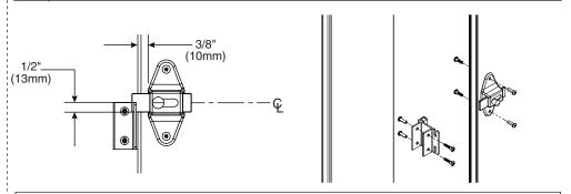
With the door in the closed position, position the strike/keeper on the pilaster and align the top so it is 1/2" (13mm) above the bottom of the latch slide bar. Using the strike/keeper as a template, mark the hole locations and drill Ø1/4" holes through the pilaster. Secure the strike/keeper to the pilaster with the #10-24 x 3/4" barrel nuts and #10-24 x 1" shoulder screws provided.
