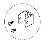
Secure the stirrup brackets to the pilasters using the #14 x 5/8" screws provided.
