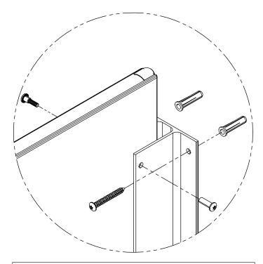
Insert plastic anchors in all holes and secure bracket to the wall with the #14 x 2" stainless screws provided.
