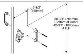
Position the wall bumper 3" (76mm) up from the bottom and 3" (76mm) from the latch side of the door (bumper goes on the outside face of the door). Using the bumper as a template, drill (2) Ø9/64" pilot holes through outside face of the door only and secure to door with the #10 x 5/8" screws provided.
