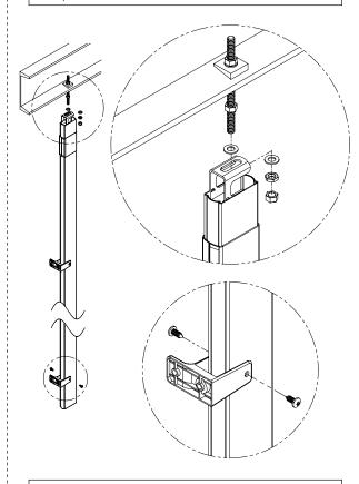
Using the bracket as a template, drill Ø3/16" holes through the pilaster at each pilaster bracket hole. Secure the pilaster to the bracket using the #14 x 5/8" screws provided.
