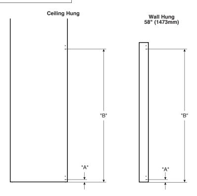
For 58" wall hung pilaster, establishing dimensions "A" and "B" as shown in the table will result in the top of the door being flush with the top of the pilaster when the cam setting on the door is set to  $0^{\circ}$ .
