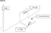
Secure bracket to wall using 1-1/2" Torx screws.
