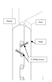
holes 3/4" deep. Install 1" Philips head countersink screws into each hole on the hinge.
