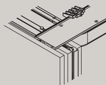
Component of the HAWA-Folding Concepta 25 set: well-thought-out connection profiles for cabinet body and sides ease the installation of overlying cabinet doors.
