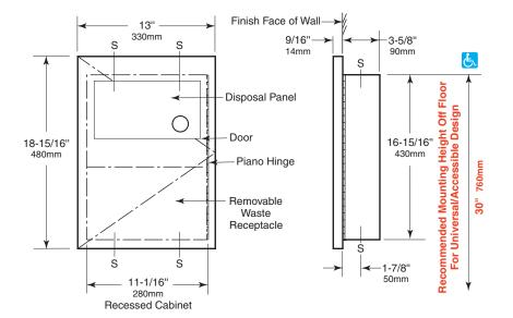
Rough Wall Opening 11-1/2" (290mm) wide 17-1/4" (440mm) high 3-3/4" (95mm) minimum recessed depth
