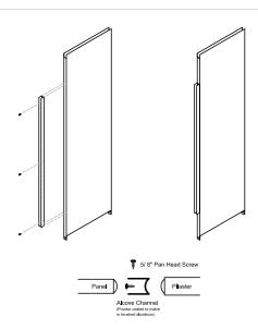
6. Attach Alcove Channel to Middle Pilaster Position alcove channel 305mm (12") from bottom of pilaster. Concave side of alcove channel mounts to pilaster. Secure with a minimum of three screws.
